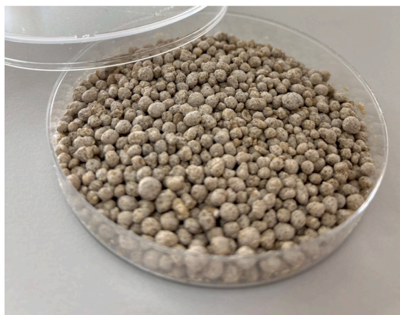
Fig. 1. The PHA-controlled release urea fertilizer (PHA-CUF).
