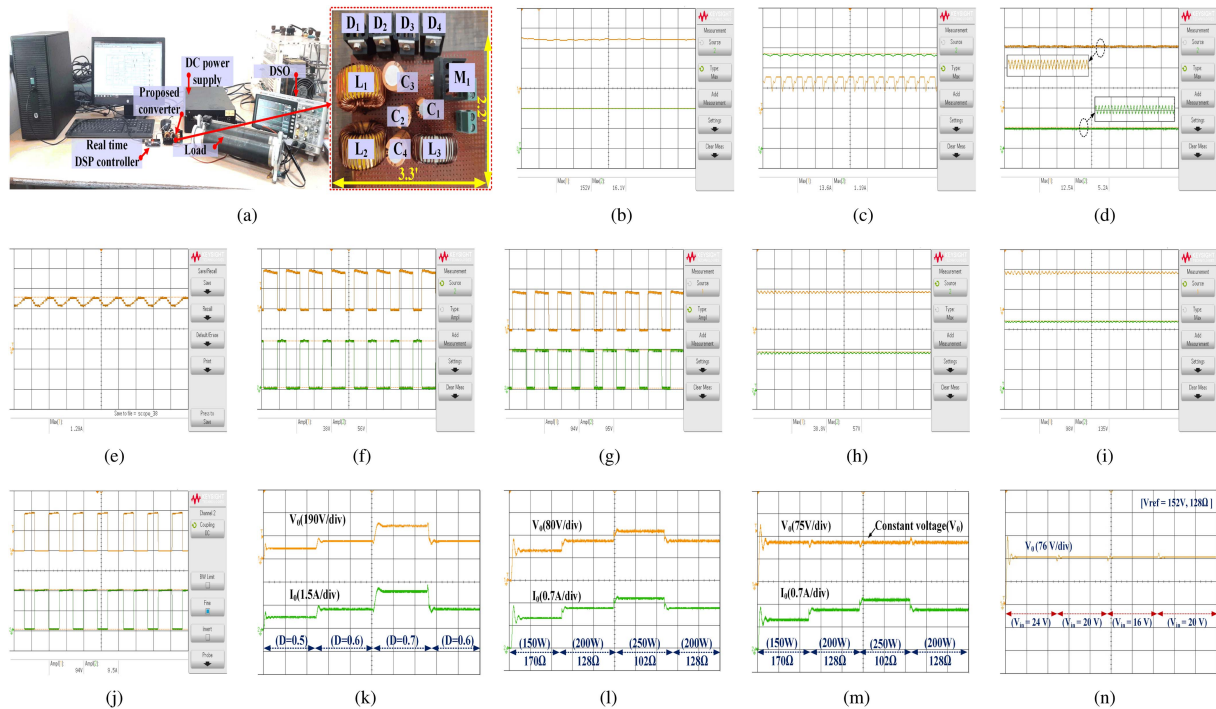
Fig. 8. (a) Experimental set-up of the proposed converter. (b) V_i & V_o . (c) I_{in} & I_o . (d) I_{L2} & I_{L1} . (e) I_{L3} voltage across (f) D_1 & D_2 , (g) D_3 & D_4 , (h) C_1 & C_2 , and (i) C_3 & C_4 . (j) Voltage and current across switch M_1 . (k) V_o and I_o for changing the duty cycle with 128 \Omega . (l) V_o and I_o for changing the load values at 60 % duty cycle. (m) V_o and I_o for changing the load values at constant input voltage in closed-loop. (n) V_o for change in input voltages at constant load in closed loop.
