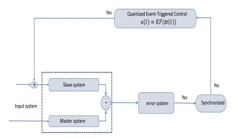
**Figure 2.** The flowchart of the proposed controller in Example 1.
