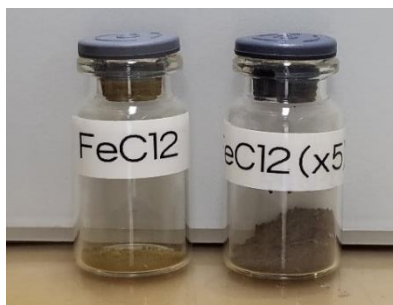
Figure 1. Sample color comparison between batches prepared under ambient conditions (left) and in an anaerobic glove box (right). The sample not exposed to oxygen shows a darker color.
