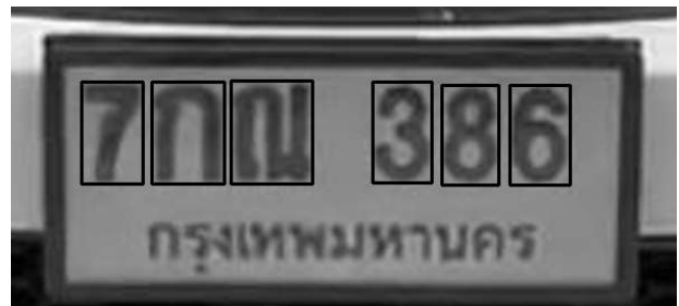
Fig. 9. Filter out unwanted contours
