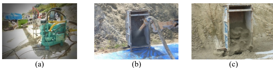
Figure 5: Preliminary test on ground surface. (a) Layout of preliminary test on ground surface; (b) Spraying the buffer material with 14% water content; and (c) Spraying the buffer material with 18% water content.
