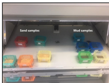
Figure 7: Samples mixed in mud and sand placed in the UV weathering chamber for further conditioning.
