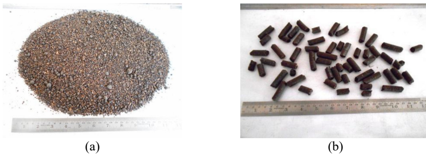
Figure 2: (a) Sample of dry olive pomace; and (b) Pelletized dry olive pomace.
