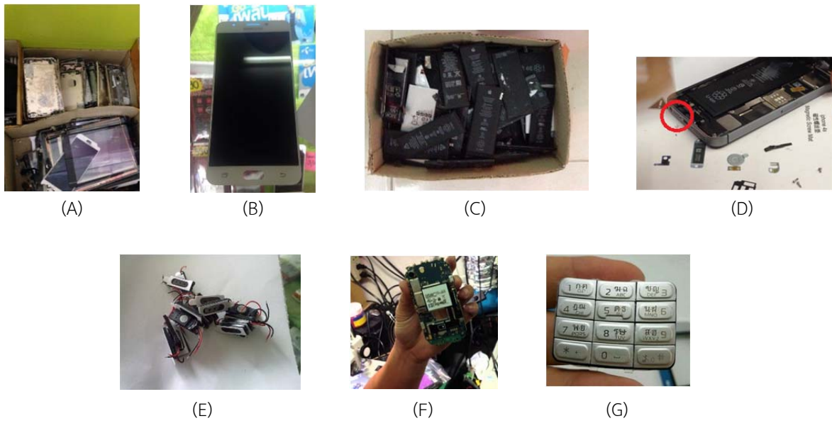
Figure 1 Type of mobile phone waste (A) Phone mask (B) Liquid crystal display (C) Batteries (D) Speakers (E) Microphone (F) Circuit board (G) Keypad
