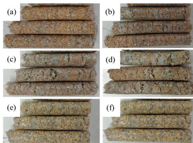
Figure 2 Non-torrefied and torrefied pellets of (a, b) PET/TS, (c, d) PET/ES, and (e, f) PET/CC
