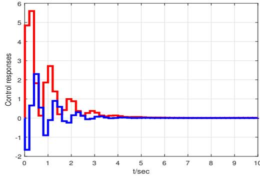
FIGURE 2. Trajectories of control input for the Example 5.1 with  $L_2$ - $L_\infty$  performance
