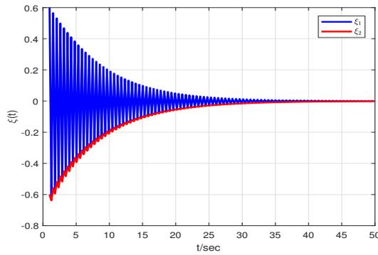
FIGURE 12. State responses of the system with (43)  $(Q, S, R)$ - $\gamma$  Dissipativity performances
